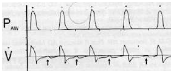
Figure 1. Airway pressure (PAW) and flow (V) tracings in an intubated mechanically ventilated patient. Nota asynchronous spontaneous respiratory efforts (arrows) during machine deflation. (Dots: mechanical inflation)
